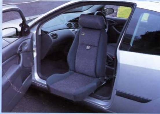
Seat rotated and extended to make access much easier!
