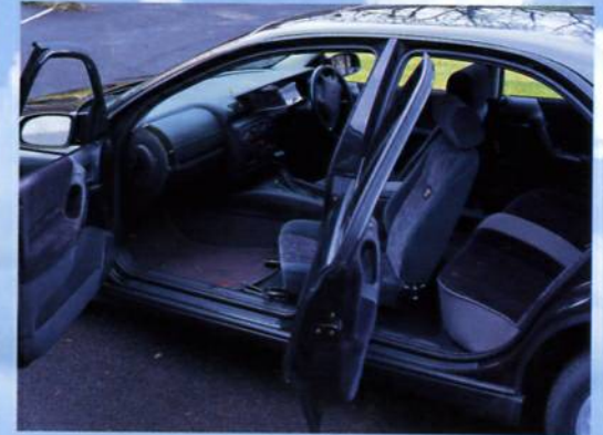
Seat slid fully rearwards to achieve maximum leg clearance during seat rotation.
